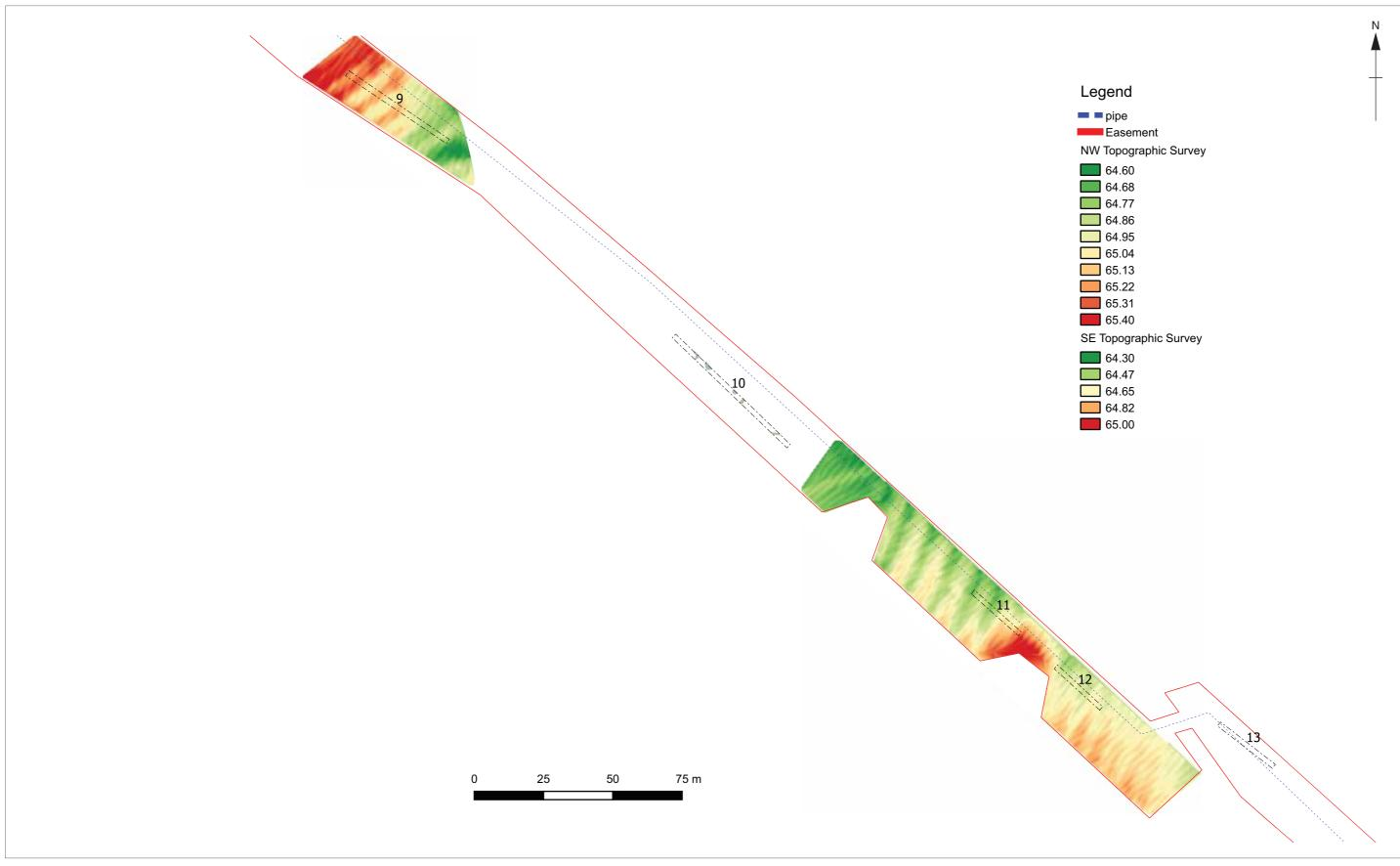
Figure 6: Topographic Survey showing ridge and furrow
